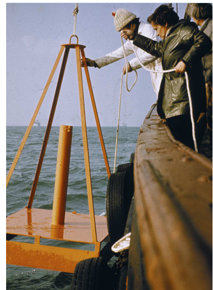
Figure 9: Typical Mary Rose Transponder Frame. (BP)
