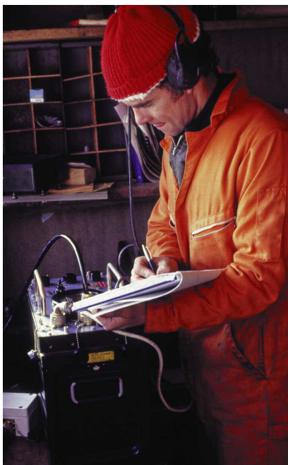
Fig 15: Mary Rose diver with Remote Transducer connected to LBL Transceiver. (Nick Rule)
