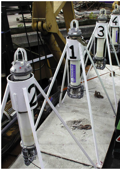
Figure 29: Mk4 Compatt Transponders mounted in Seabed Frames. (Author)
