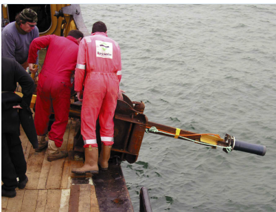
Figure 35: Deploying the Scout USBL transceiver from Terschelling. (Author)
