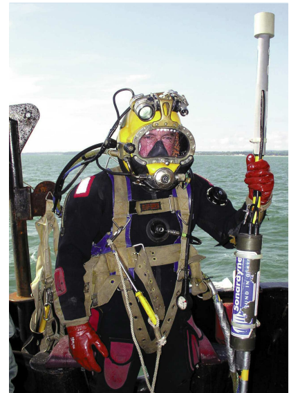
Figure 28: Diver holding survey staff fitted with a Mini RovNav transceiver. (Author)
