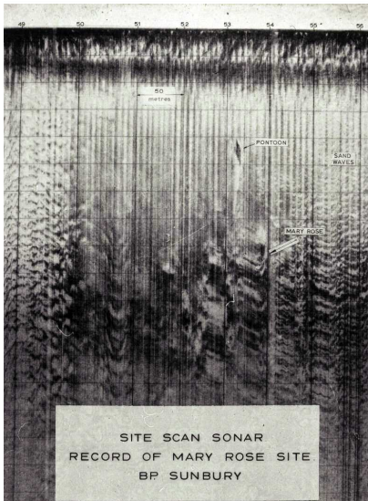
Figure 4: Side-Scan Sonar Plot. (BP)
