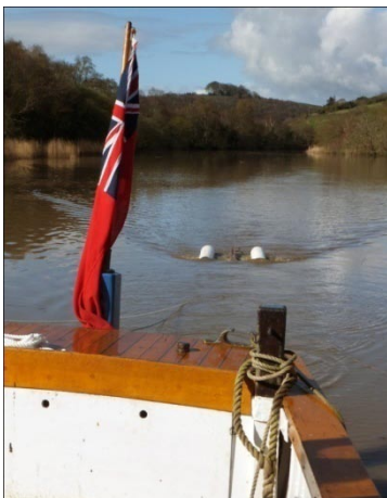
Towing a side scan sonar on the Tamar near Calstock
